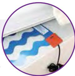
Epilepsy sensors are used to monitor people with epilepsy while they sleep. Patented sensor technology detects a person's movement in bed and is able to differentiate normal movements from epileptic seizures.
