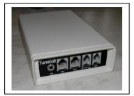
The Wandering Client Sensor provides a facility to monitor for potential wandering situations. Should the system believe that a wander event has occurred an alarm is automatically raised. An alarm will also be raised if the door being monitored has been left open.
