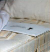
**Bed occupancy sensor** an under-mattress pressure pad which raises an alarm if the user has left their bed and not returned within a pre-set time period.
